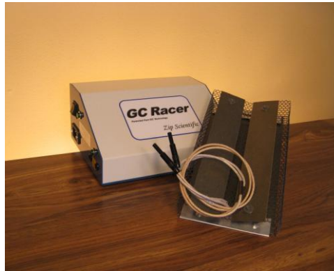
Figure 1 GC Racer: control box and auxiliary heater
