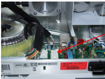
7890 - 1 Remove the back panel & unplug the 2 transformer connectors.
